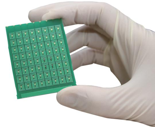
→ A semiconductor bio-sensor system that can detect AI virus in the field quickly and with high sensitivity.
