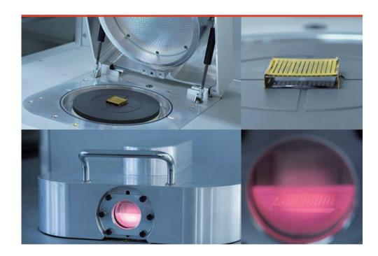
Here, we introduce a generalized method for creating perpendicular orientations by filtered plasma treatment of the BCP films. By cross-linking the surface of disordered BCP films using only physical collisions of neutral species without ion bombardment or UV irradiation, neutral layers consistent with the BCP volume fraction are produced that promote the perpendicular orientations. This method works with BCPs of various types, volume fractions, and molecular weights
