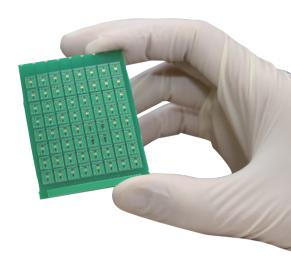
A semiconductor bio-sensor system that can detect Al virus in the field quickly and with high sensitivity.
