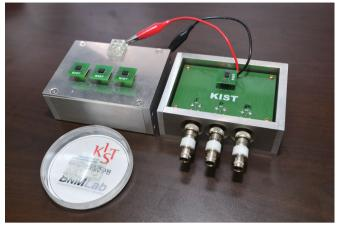
The highly sensitive Al virus detection diagnostic platform, allows for immediate analysis of samples taken from the field.
